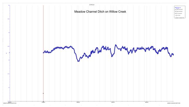
Note: Recorder was placed at the land intersection of the California Department of Fish and Wildlife and the Hanson ranch. A measure of depth is not a reflection of the flow of the system. All depth measurements are relative to a starting measurement on 7/11/2022, a negative value represents a depth below that reference measurement.
